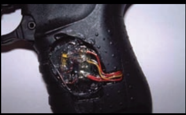
Figure 7: Force sensing resistors embedded in the handstock. The sensors were subsequently disguised.
